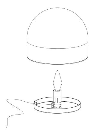
**3** Secure the shade to the base using the 3 screws supplied.
