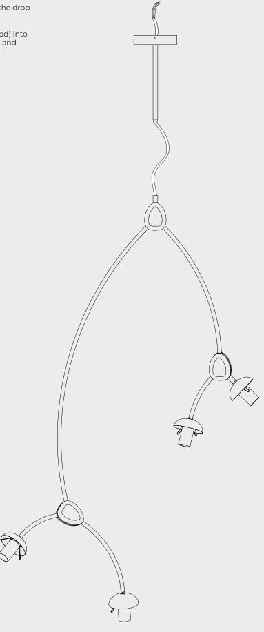
Raise the pendant and make the electrical connections ensuring all wires are colour matched and the pendant is earthed correctly.
