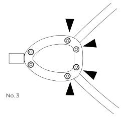
**3**. A. Feed the power cable from hub through the droprod and into to the ceiling rose cover.
