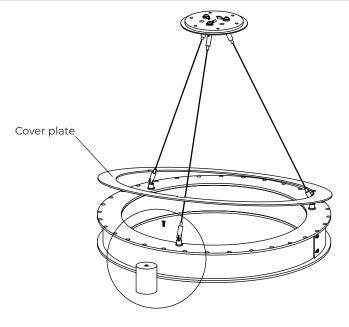
**3**. Set to correct desired height, make sure fitting is level using a spirit level. Critical, do not let fitting hang unbalanced. Make note of minimum height of fitting.
