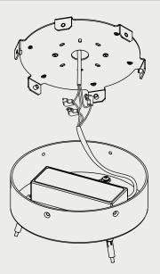
**3.** Bring the ceiling rose cover up to the mounted plate and secure with the six screws.
