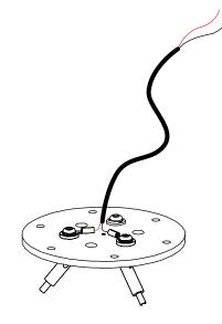
**3.** Mark out fixing hole, and use suitable fixings for the fittings weight. x6
