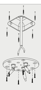
4. Attach to ceiling and install cover plate, with M3 screw.
