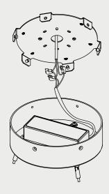
Bring the ceiling rose cover up to the mounted plate 3. and secure with the six screws.
