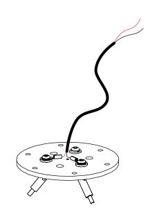
230V Mark out fixing hole, and use suitable fixings for the fittings weight. x6 (not supplied).
