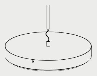
**2.** Place the ceiling rose onto of the drop rods and attach using the supplied washes and nuts.
