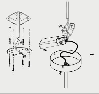
A. Make power connection to the LED driver. See wiring diagram. Place driver inside ceiling rose.
