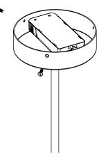
6. Bring the fitting up to the ceiling plate, to attach.
