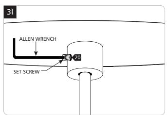
20 Make any fine adjustments necessary then secure the fixture wires in place with the set screw and allen wrench.
