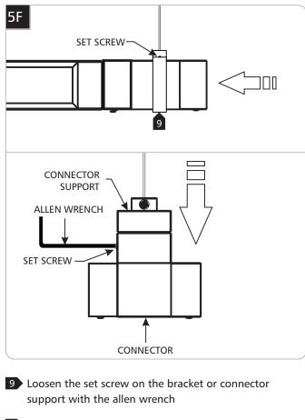
Slide bracket from the previously installed supports over the connector or insert the connector support into the connector.
