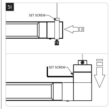
**16** Slide the support bracket over the end cap or insert the connector support into the connector.
