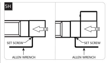
For open ended systems, slide the end cap or connector onto the light bar.
