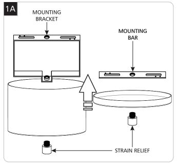
Unscrew the strain relief from the canopy to remove the mounting bar/bracket(depending on your canopy type).
