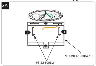
Secure the mounting bracket to the junction box with #8-32 screws.
