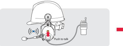
First, connect the two-way radio cable with the headset.
