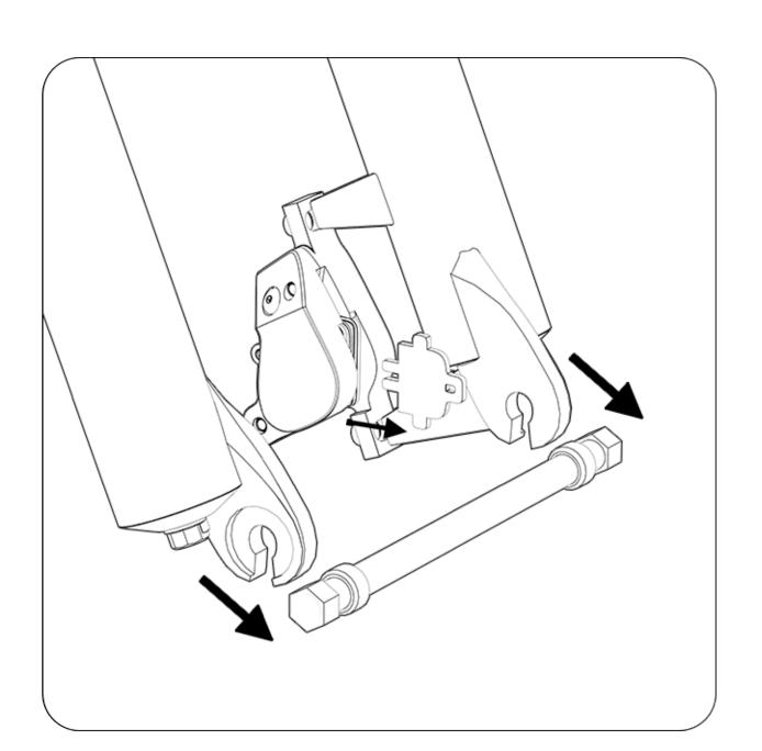
3. Remove the front fork protective rod and brake protective pad.
