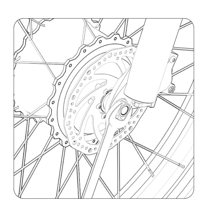
8. Use a wrench to tighten the screws.
