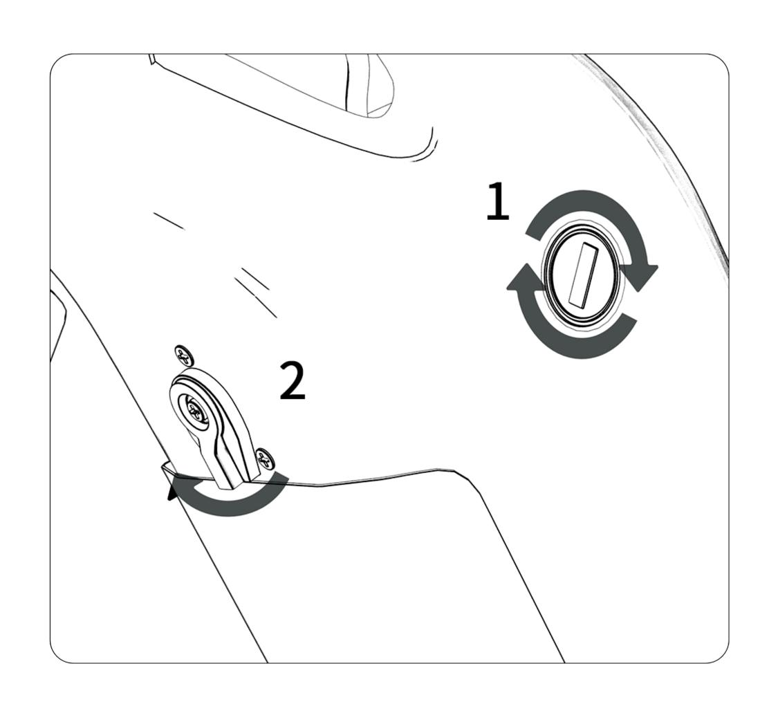
1. Unlock the battery with the key
