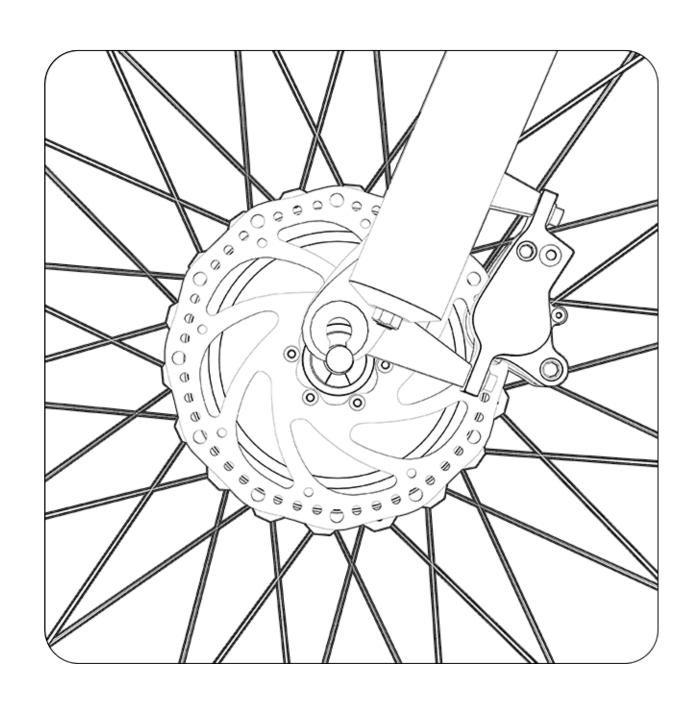
6. Front fork alignment motor shaft installation.
