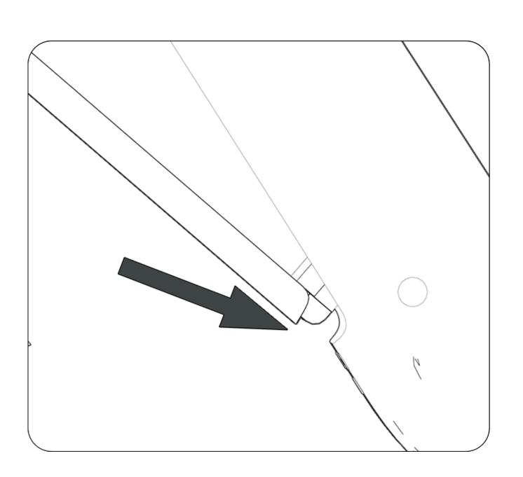
1. Install the battery with the contact side down.
