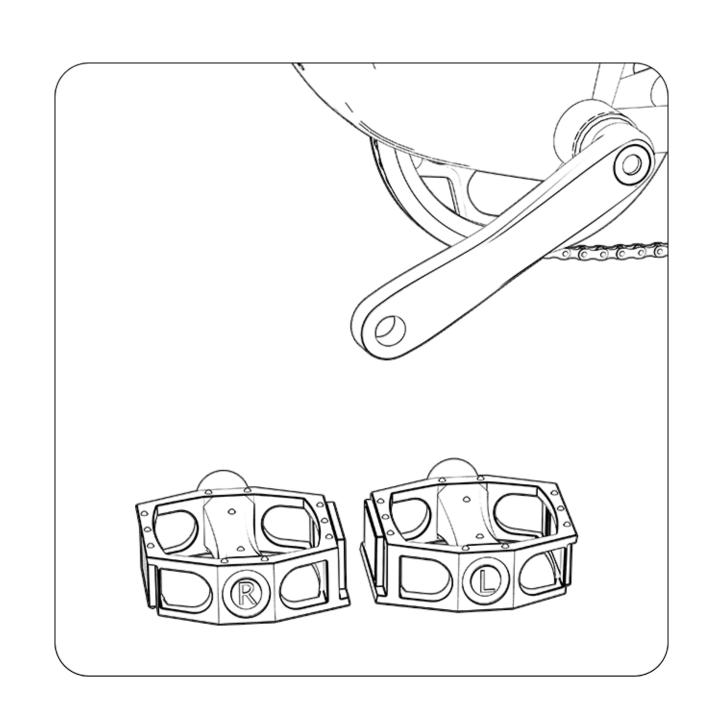
11. When installing the foot pedal, pay attention to distinguishing between "R" and "L".
