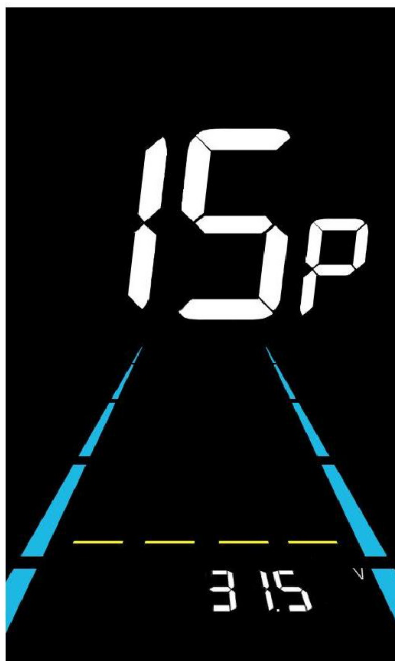
image 6-15 Battery under-voltage value setting interface.
