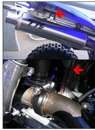
frame above the muffler. Slip the stock pipe off, (you may want to keep it in the box in which came our Slip-On pipe for protection in storage.)
