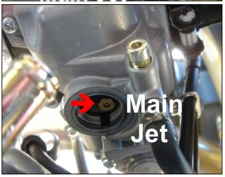
The Main Jet will be exposed in the center of this hole. The Main Jet is the brass hex-shaped jet right in the middle of the hole. Using a 6mm wrench or socket, remove the Main jet and replace it with the included #180 Main Jet we supply.
