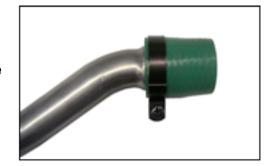
You might want to use a longer bolt for this as the stock one might be a little short. Now you can align and tighten the green silicone seals over the connection of pipe and stinger. Center the Green Seal tube so that both clamps will be on either side of the joint seam so the clamp will snug down on the rubber.
