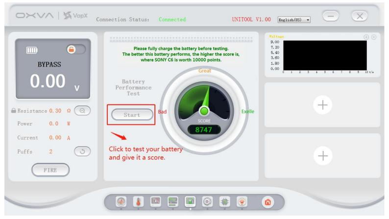
Noted: The device will quickly ignite twice and give the score when start. Batteries with a score below 2000 will be notified that they cannot be used. The rate is based on the battery's current, internal resistance and performance of the cell.
