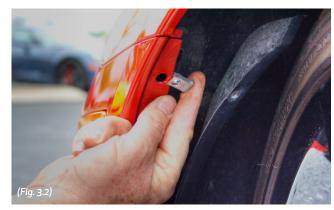
**Note:** the pin is a male/female assembly. The male piece can be pried loose from the female piece using a flat blade screwdriver. Insert the blade of the screwdriver in the slot at the edge of the pin and twist the screwdriver causing the pin to come free of the female piece. After removing the male piece, the female piece can be easily removed.
