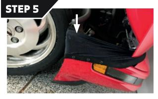
Begin the installation of the mask by fastening the top snap on one end of the mask to the snap-head screw installed at the top edge of the bumper.
