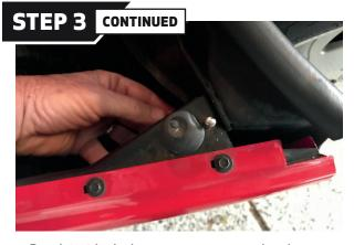
Reach inside the bumper to remove and replace the U-clips at the edge of the bumper.
