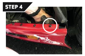
On the top edge of the bumper, remove and replace the OEM screw located in the first horizontal position adjacent to the wheel well with supplied snap-head screw. It is not necessary to remove the U-clip that secures this screw.
