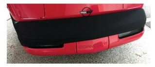
Stretch the mask across the front of the bumper and attach to the other side of the car. (Note: the bottom of the mask can be identified by the label located along the bottom edge of the mask.)
