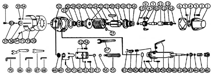
OILING INSTRUCTIONS: OIL AFTER EACH USE WITH A FEW DROPS OF AIRTOOL OIL THROUGH THE AIR INLET. RUN FOR ONE SECOND TO COAT ALL INTERNAL PARTS.
