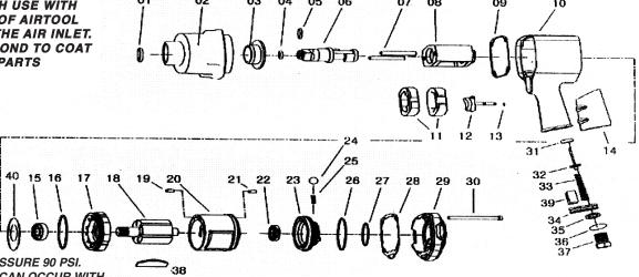
USE MAX. AIR PRESSURE 90 PSI. CLUTCH DAMAGE CAN OCCUR WITH HIGHER PRESSURE.
