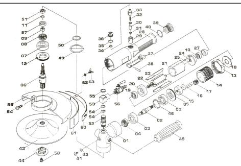
**OILING INSTRUCTIONS:** OIL AFTER EACH USE WITH 1/2 TEASPOON OF AIRTOOL OIL THROUGH THE AIR INLET. RUN FOR ONE SECOND TO COAT ALL **INTERNAL PARTS**
