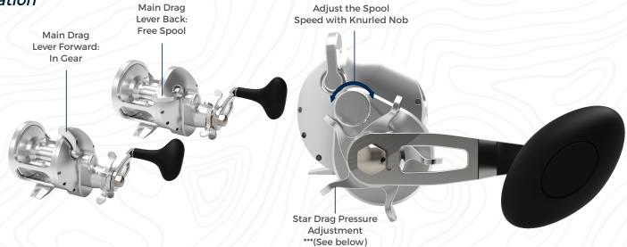
Adjusting the spool speed with knurl spool knob, you should tighten it all the way and put reel in freespool. Let the bait or lure hang off rod tip and slowly turn knob backwards until lure or bait slowly falls. This is a good setting to start and if you feel like you need freer spool continue to turn knob backwards till you feel its set appropriate for your casting needs.
