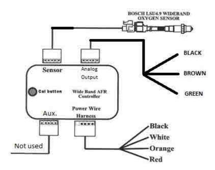
Parts included: Bosch LSU4.9 Oxygen Sensor Sensor wiring harness Stainless weld in bung
