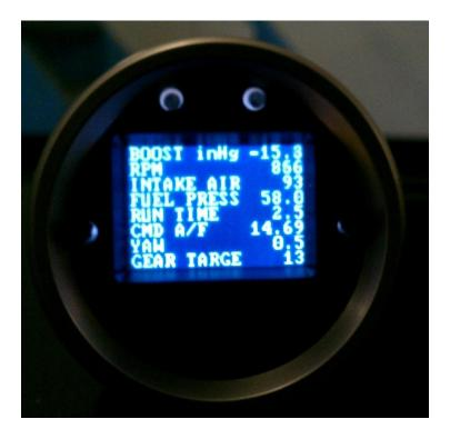
This screen will display the 8 parameters chosen in **Cyclic Scan**, or the two parameters that were last displayed in normal **Scan** mode plus the last 6 in **Cyclic Scan**.
