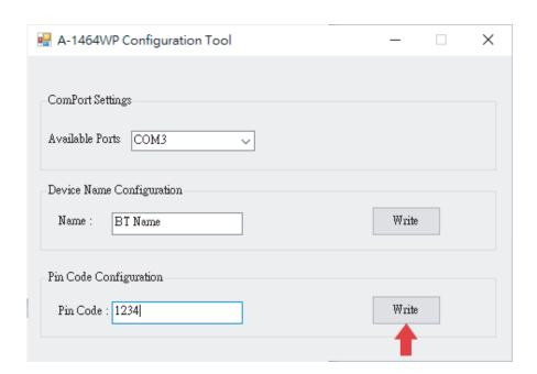
STEP9: Confirm the Bluetooth Pin Code with Smartphone. If Pin Code is not changed. Make sure USB TTL Cable is connected to the Micro USB Port on the LB-BTAMP5 and go back STEP7 – STEP8
