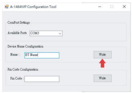
STEP6: Confirm the Bluetooth Device name with Smartphone. If name is not changed. Make sure USB TTL Cable is connected to the Micro USB Port on the LB-BTAMP5 and go back STEP1 -STEP5
