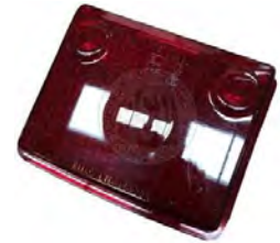
Stop/Tail Lens for Combination Lamp
