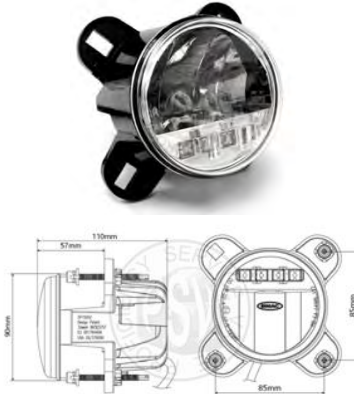
LED 90mm Main Beam Headlight with Integral Position Light
