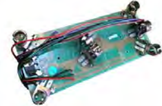
6 Pin Plug Assembly for Combination Lamp
