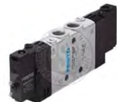
24V 5/2 Way Double Solenoid Valve, Bistable, 1/8" Pneumatic Connection
