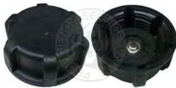
Cap with valve, expansion tank
