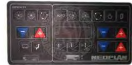
Heater Control Panel
