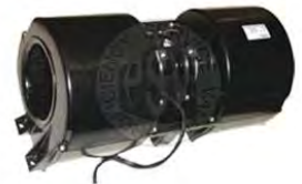
Twin Blower 24V 1100 m3/h Airflow Width: 80mm, Height: 170mm, Length: 465mm
