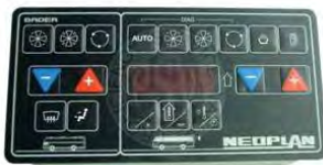
Heater Control Panel
