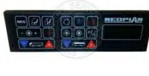
Heater Control Panel
