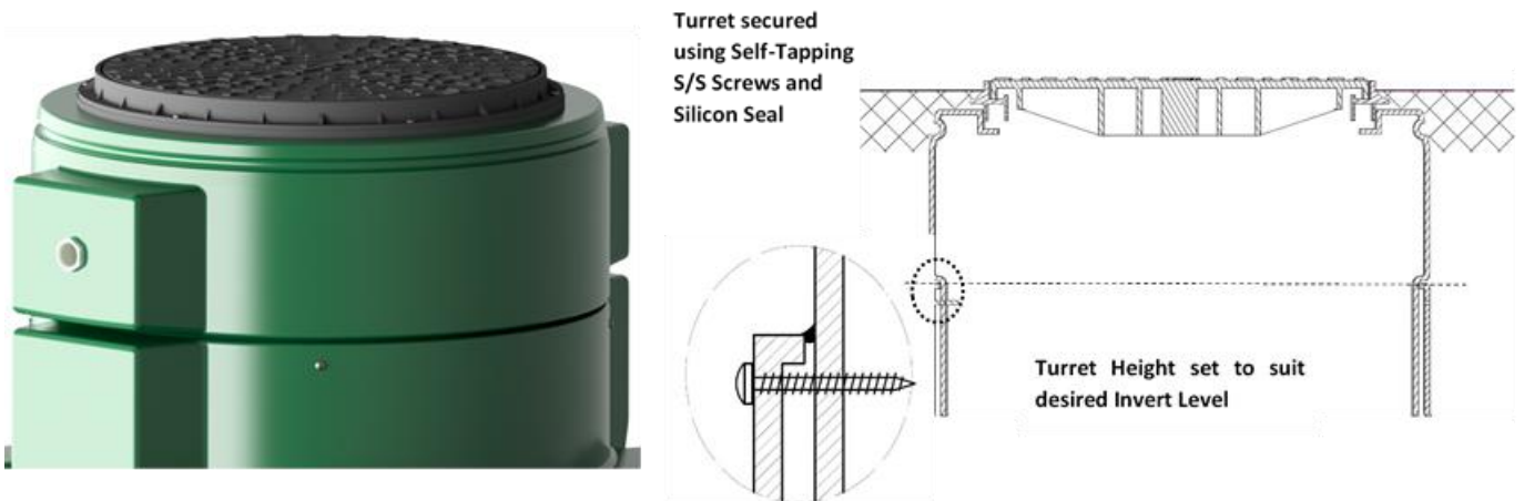
Figure 8: Reduced Turret Height Image and Modifying the Tank Invert Level
