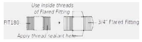
Then, connect the FIT180 fitting into the coupling located on the bottom of the aluminum plate. Tighten.
