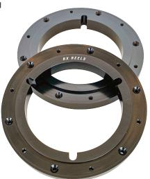
The flanges are secured to either side of this NAB hub. which is machined out of solid aluminium to RX Reels' specifications. In contrast, most NAB hubs are plastic mouldings. Manufacturing tolerances for this 23-gram hub are claimed to be "below two thousands of an inch". Twelve countersunk screws keep the lightweight but strong carbon-fibre flanges in position.
