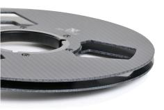
The flanges of RX Reels, which have a thickness of just over 2mm, are made from upcycled aerospace-grade carbon fibre for toughness and longevity. They don't warp and are resistant to bending. The iconic 'Technics-pattern' cutouts, made using a highpressure jet of water under computer control, were chosen because they "make tape threading easier".
