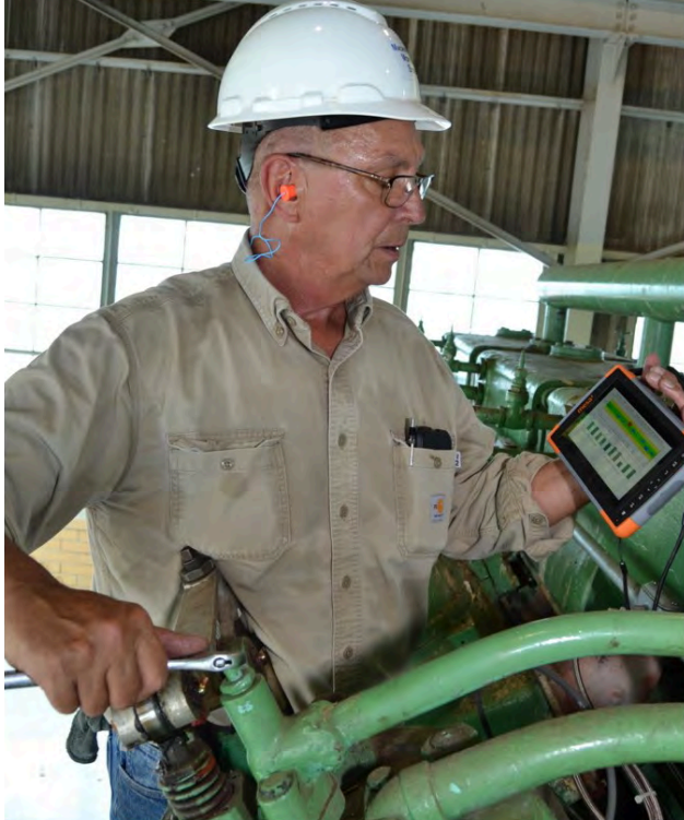
A technician is using ProBalance with a tablet to balance an engine.
