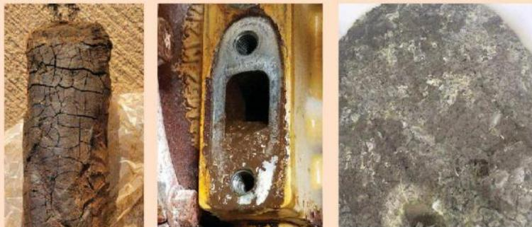
(Left To Right) A filter from a Caterpillar 3516 has been gummed up with phosphates after running detergent/Cascade in the cooling system. Phosphates can be seen congealing after running detergent/Cascade in the cooling system. Drained PO4 Fix After Running Four Hours At Temperature
