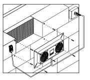
4. If the mounting board needs to be modified to accommodate important openings, the following trimming advice should be followed: be careful when trimming the mounting board to avoid damage to the power cord.
