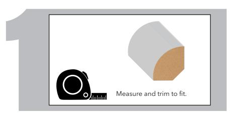
Leaving a 1/4" space between flooring and the wall, cover the gap with quarter round molding. Laminate Floor
