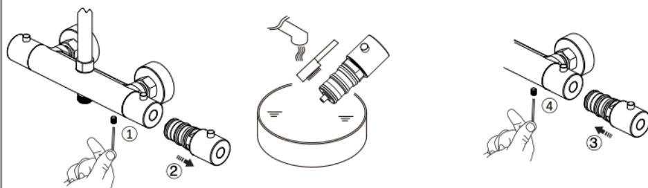
**Vervanging thermostatisch element****2***Replacing the thermostatic valve core*
