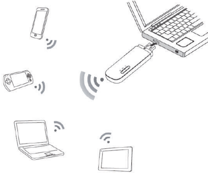
Figure 3-2 shows multi-devices access the wireless work through Wi-Fi and USB.
