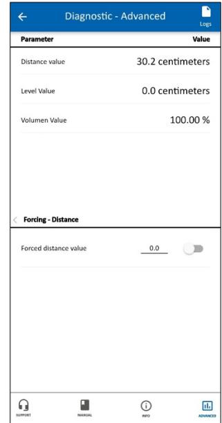
Figure 30 – Forcing: Analog Output
