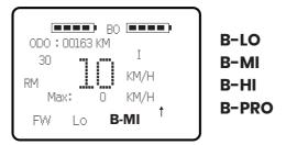
Pull the Throttle Wheel back on the remote control and do not release it. At the same time, short press the (2) to switch the four gears of the braking strength.
