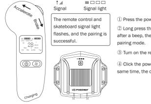
① Press the power button 创 of the skateboard to turn on. ② Long press the power button 创 for 5-7 seconds, after a beep, the signal light flashes to enter the pairing mode.
