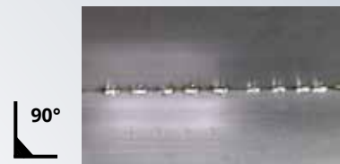
Corner spot welding thickness 0,6 mm
