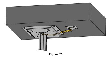
**13B]** For truss mount: Use a quick link to secure one end of the safety cable 12 around the truss. Conduit the other end of the safety cable 12 into the upper tube 2 and lower tube 3, as shown in Figure 88.
