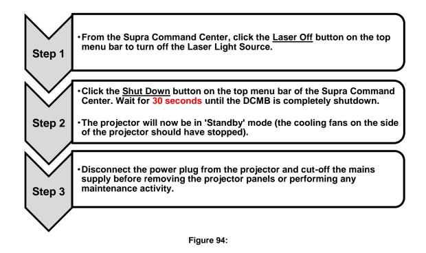
Please Note: When the Supra-5000 is in 'Standby' mode, you can access the Supra Command Center web interface using the URL: <u>http://192.168.254.241</u> and click the **Power On** button on the top menu bar to boot-up the DCMB Web UI.
