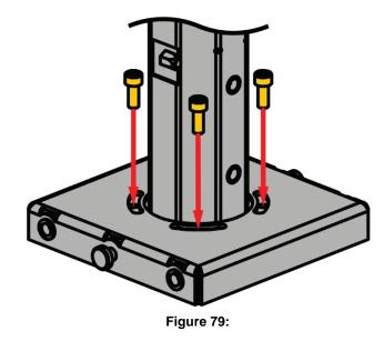
Step 5: Tighten the top plate 4 to the lower tube 3 using the bolts 8 (4 pcs.), as shown in Figure 79.
