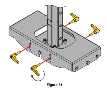
**Step 7:** Tighten the middle plate (5) to the top plate (4) with the help of the clamping handles (9) (4 pcs.), as shown in **Figure 81**.
