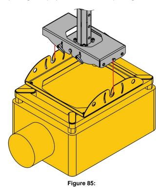
Step 11: Attach the projector plate (6) and projector to the middle plate (5), as shown in Figure 85.
