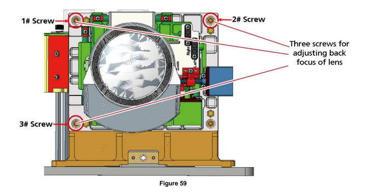
**Step 3:** Observe the clarity of different areas of the picture. If the clarity of the whole picture is consistent, there is no need to adjust the back focus. If the picture has up and down pitching, adjust by adjusting **1# and 2# screws** at the same time or adjusting **3# screw** separately. If there is left-right pitching, adjust it by adjusting **1# and 3# screw** or adjusting **2# screw** separately until the global picture is clear.
