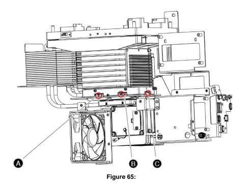
**Step 4**: Project a grid test pattern. When the Red grid and the Cyan grid do not coincide, adjust the knob screws **A**, **B** or **C** to adjust up/down, rotate and left/right.
