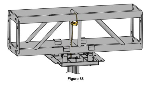
**Step 14:** Attach the other end of the safety cable (12) to the projector plate (6) using a quick link, as shown in **Figure 89**.
