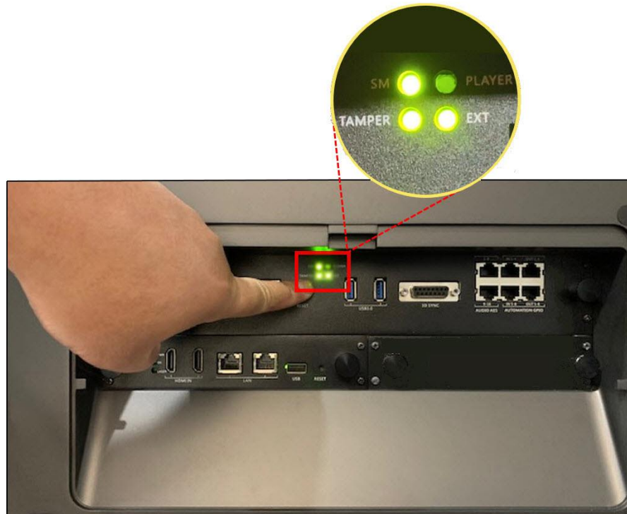
Figure 4: Working status of SM, TAMPER and EXT LED Indicators on the DCMB
