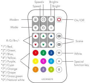
Mode+/-: Short press switch dynamic mode built in controller, long press 2s Mode+ run mode cycle, long press 2s Mode- run the first mode.
