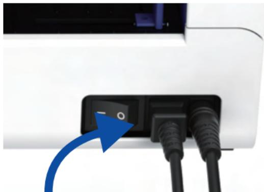
4. Turn the power ON (Press down "-" means Power ON), now you will see the top feeder button flashing.
