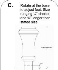
Optional: For additional support, foot can be secured to floor. Screw nylon bushing into desired location on floor.
