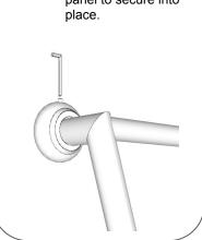
D. Rotate at the base to adjust foot. Size ranging ½" shorter and ¾" longer than stated size.
