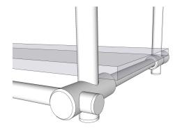
B. Mount collars to surface blocking or ceiling blocking and affix by screwing into place.
