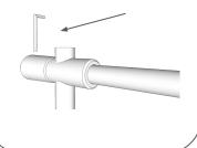
F. Insert the horizontal rod into the bottom fitting and secure with set screw. Place desired shelving onto brackets.
