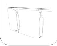
E. Once all pieces are in their final position and level, tighten all connections. Slide foot rail pieces into brackets and tighten with provided set screws.
