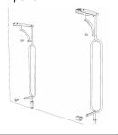
Install top angle iron pieces and decorative end pieces using supplied hardware, making sure it is level. Make any adjustments for feet at this time.
