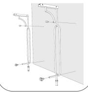
B. Place two 5/16" nuts onto the supplied rail bolts to drive the bolts into the wall studs/blocking. Leave 2-½" length from wall for top bolt and 5-½" length for bottom bolt.
