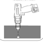
\*Optional: Foot sleeve fits over nylon bushing to secure to floor.
