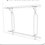
\*Optional: For additional support-foot can be secured to floor. Screw nylon bushing into desired location on floor.
