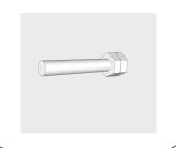
Remove 5/16" nuts from bolts. Slide supports onto exposed bolts. **DO NOT** fully tighten purse hook or foot rail bracket at this point.
