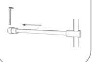
E. Insert the horizontal rod into the bottom fitting and secure with set screw. Place desired shelving onto brackets.
