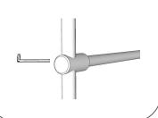
D. Slide end fittings into each mounting collar. Tighten set screw against the wall mounted fitting to secure vertical assemblies into place.
