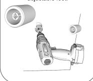
D. Make sure all set screws for vertical rods are backed out of each hole for easy assembly.
