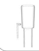
B. Mount collars to surface blocking or ceiling blocking and affix by screwing into place. Leave 3 ½" under vertical rod for adjustable foot.
