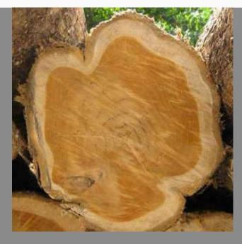
The separation between grade A and C is obvious when looking at a cross-section of a teak log (Tectona Grandis). However, it is important to note that grade C can be made to look like grade A with the use of chemicals. See "IMPORTANT" section below.
