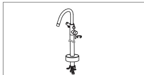
2. Match the square pole with the main body, fix together turning the 2 screws on rear with the key.
