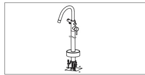
6. Insert the fixing bolts and fix tight in the floor. Move the cover to hide the base.
