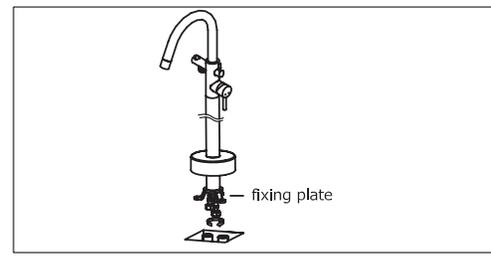
4. Insert the sliding cover on square pole, insert the flexible hose's nuts through the fixing base and connect the G 1/2 nuts with the water net connectors fixing tight by key.
