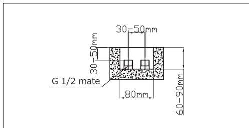
3. Create a chamber in the floor following the above measure with G 1/2 male connectors for water net.
