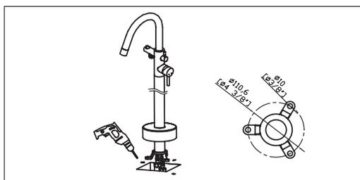
5. Adjust the complete to get correct position, then drill to fix base plate.
