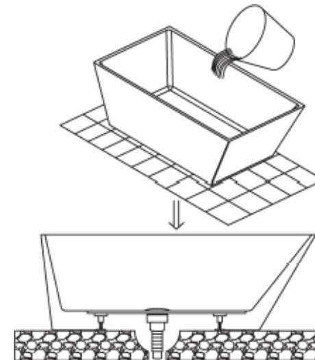
5. Apply a thick heed of silicone within bath outline allow to set 24 hours. This installation guide and the installation of waste connection should be only suitably by qualified person.
