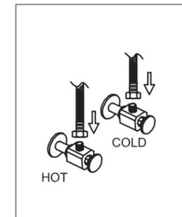
5. Attach flexible hose to water supply.
