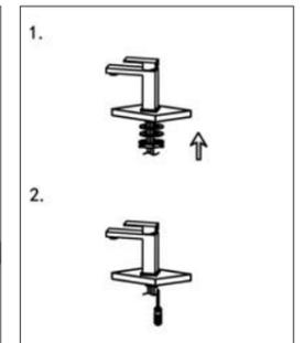
4. Re-install the rubber washer followed by the metal washer and lock-nut. Hand tighten then tighten further using a screw driver to tighten lock-nut screws.
